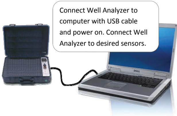
Connect Well Analyzer to computer with USB cable and power on. Connect Well Analyzer to desired sensors.
